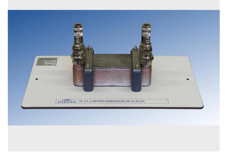
In the plate heat exchanger, the hot and cold flows alternating sides pass through the gaps left by the plates, thus resulting in heat transfer.
